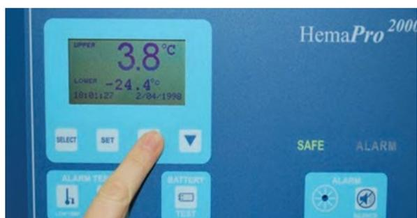
Check the temperature inside the storage unit, wait 30 minutes, without opening the door, to allow the temperature to stabilize and check it again to verify the thermostat should be adjusted.
